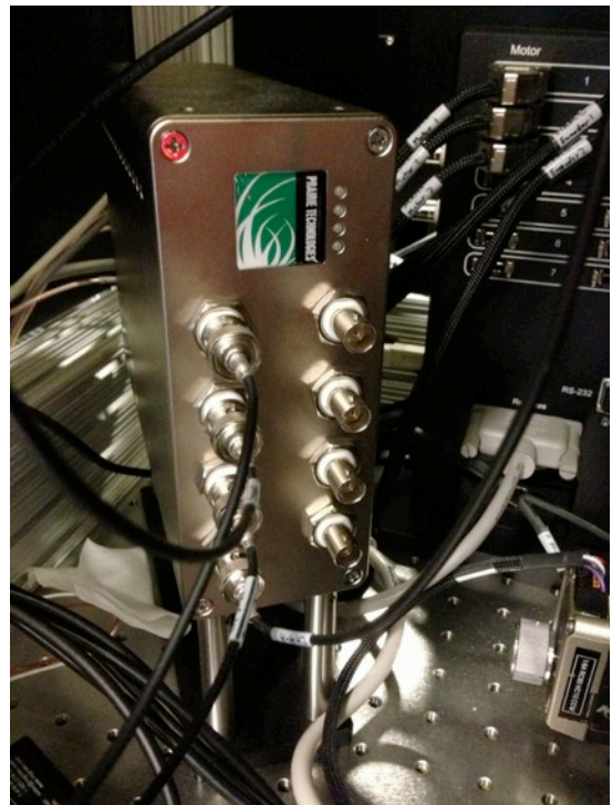
2. The Prairie PMT preamp. The inputs on the front are from the PMTs and should be left in place.
