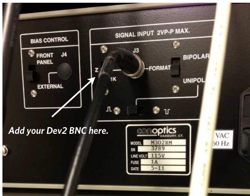
9. Back of the conoptics pockels cell control box. There are a variety of options for controlling the pockels, ScanImage and Prairie View use the same scheme so you can safely leave everything as is and just swap out Prairie's BNC with yours, or add a splitter.
