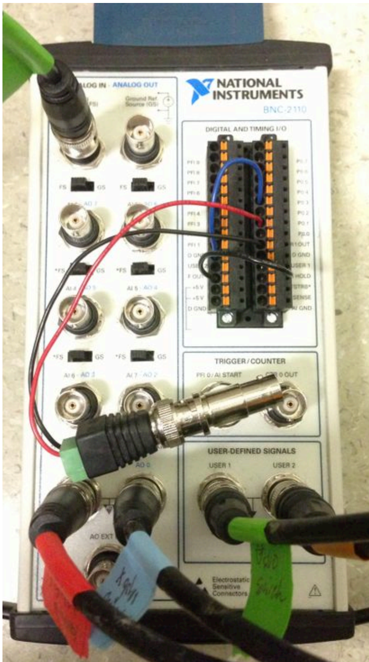
6. (above) Digital I/O organization of the ScanImage board. The blue wire routes the shutter output, which flows through P0.2, to User 2. The red and black pair, below the blue, route ground and P0.0 to a BNC connector (not shown) that is plugged into PFIO (also not shown) to route a trigger signal. The second black wire routes the +5V pin on the left to User 1 on the right.
